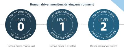
Human driver is assisted with either steering or acceleration/deceleration by the driver assistance system
